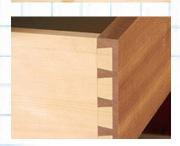
**Dovetail** - A series of 'pins' that extend from the end of one board interlock with a series of 'tails' cut into the end of another board. The pins and tails have a trapezoidal shape. Can be glued only, does not require nails. Resists being pulled apart - a strong joint.
